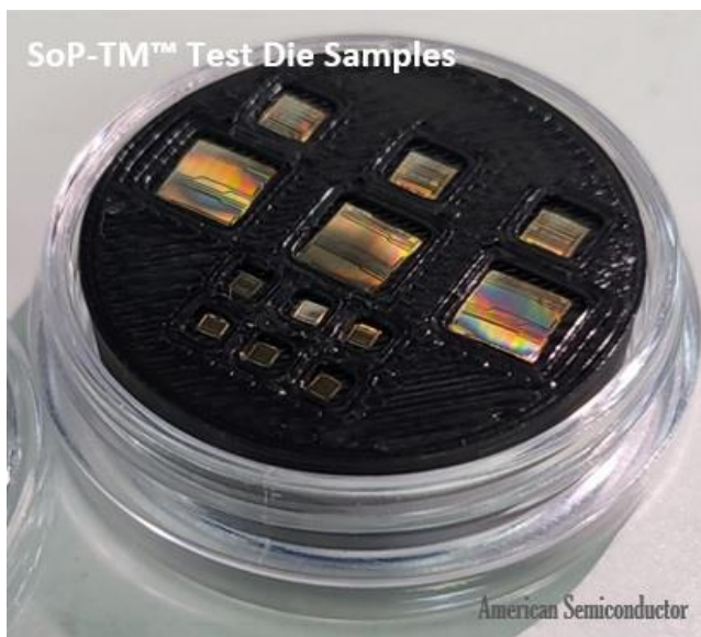
SoP-TM™ Test Die Samples in case
