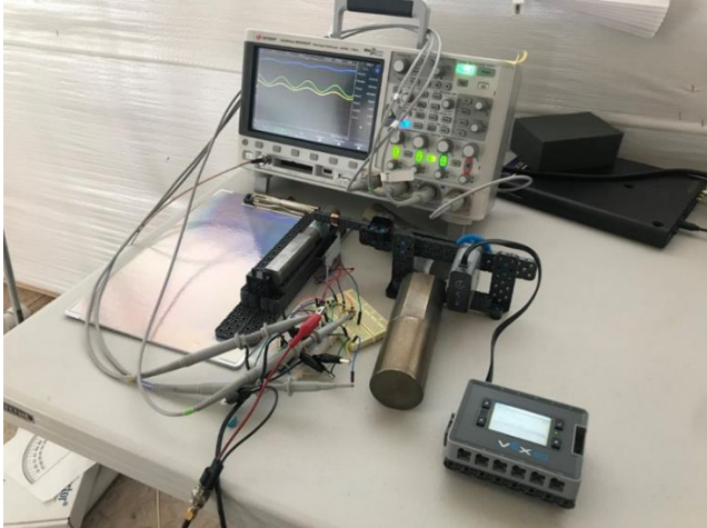
Figure 5 - OPA4002 OPAMP Set-up for reliability tests
